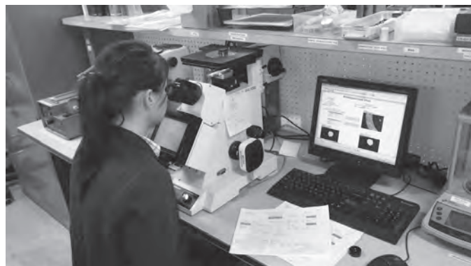
A lab service technician uses a metallurgical microscope to examine the microstructure of the metallic components in Watlow's mineral insulated metal sheathed cable, XACTPAK.
