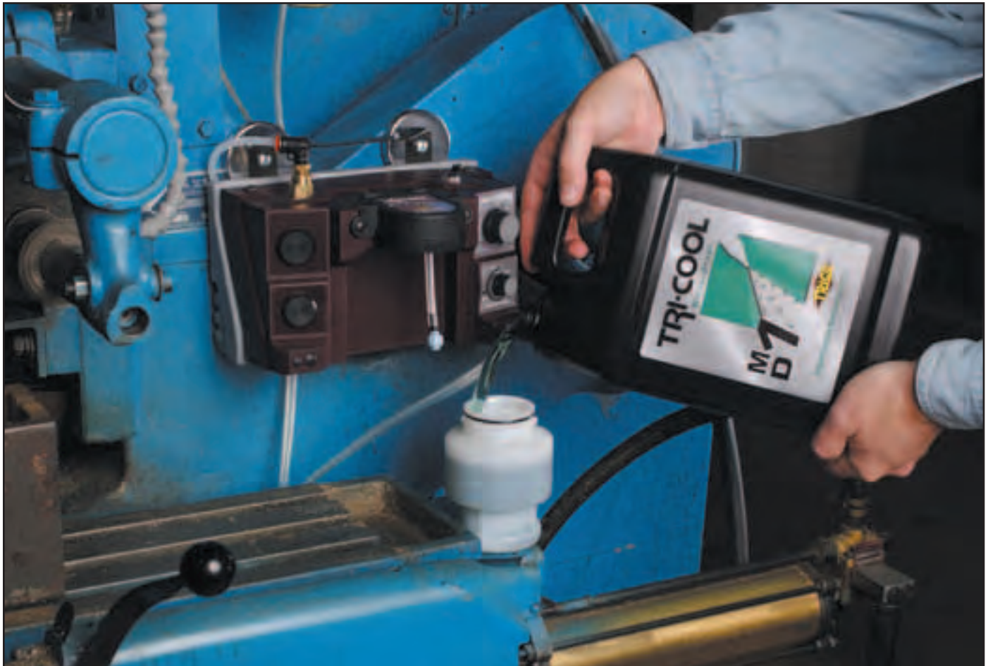
Micro-dispenser being filled with Tri-Cool MD-1 lubricant
