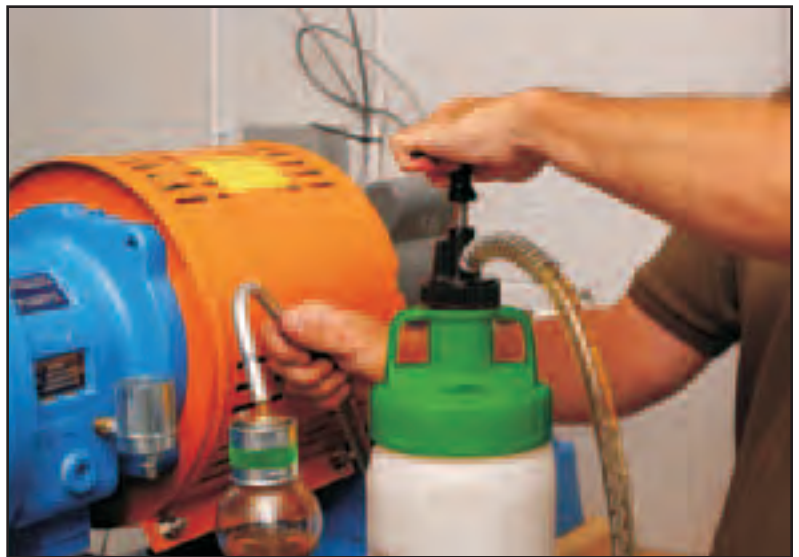
Color-coding of Opto-Matic Oilers with Spectrum Opto-Matic Collars ensures the correct lubricant is being used.
