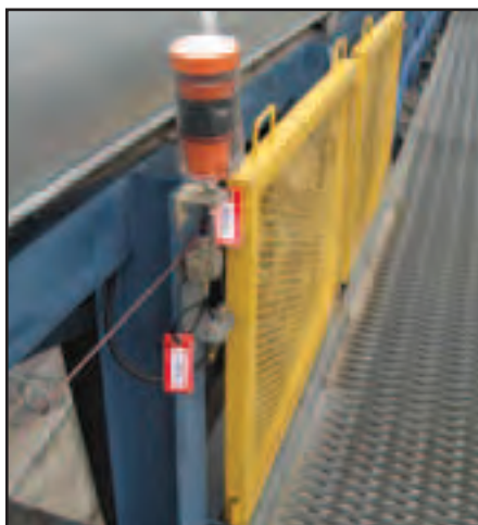
Spectrum Tags and Labels are used to identify grease lines for Automatic Grease Dispensers.
