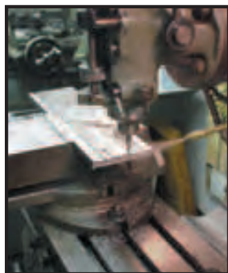
Spray cooling during milling operation
