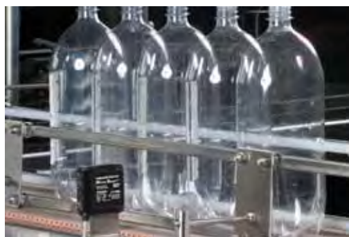
Detection of transparent PET and glass containers...full or empty.
