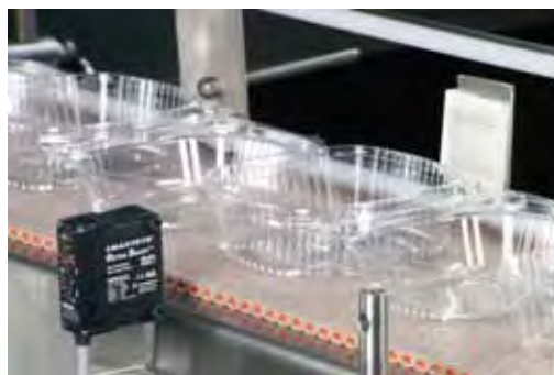
Leading edge detection of irregularly shaped objects without false signals.
