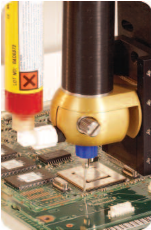
TS5000DMP - performing underfill.
