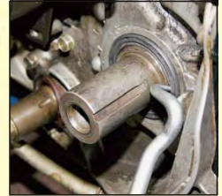
Twist and extract the seal.
