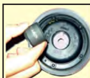
A1276 Groove nut socket to turn the camshaft adjuster into position.
