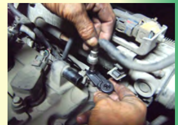
A2218 use on Injector Tube Fitting
