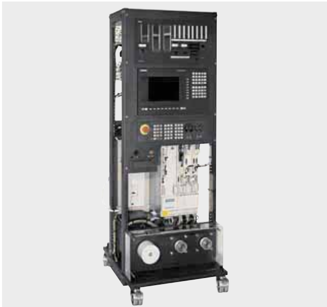
SINUMERIK 840D powerline training rack
