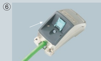
Push insert into end position. Tighten the interlocking screws of the strain-relief, push insert in, tighten jack screw
