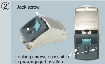
Release insert with jack screw and pull into pre-engaged position
