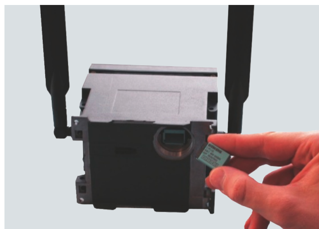
The C-PLUG is plugged into the IWLAN Access Point SCALANCE W 788-1PRO on the rear of the device
