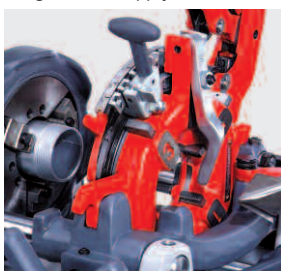
Automatic die head with integrated oil supply
