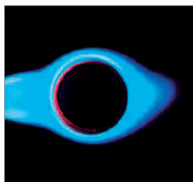
High flame temperature through cyclone swirl
