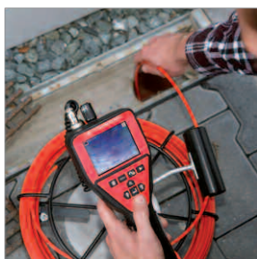
Inspection of rain drainage pipes
