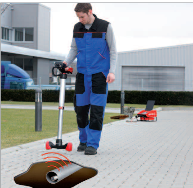
Locating of the integrated camera head with Module ROLOC PLUS
