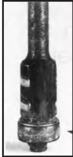
Standard flush trim router bit bearing clogged with contact adhesive.
