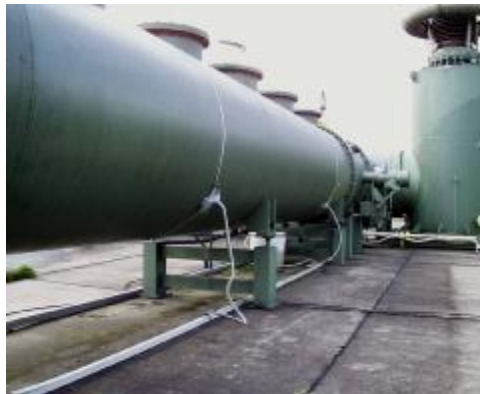
ATTanalyzer monitors a long-term test on GIS spacers and insulators (SIEMENS)
