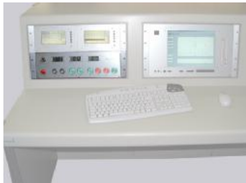
HVcontrol embedded in a control desk
