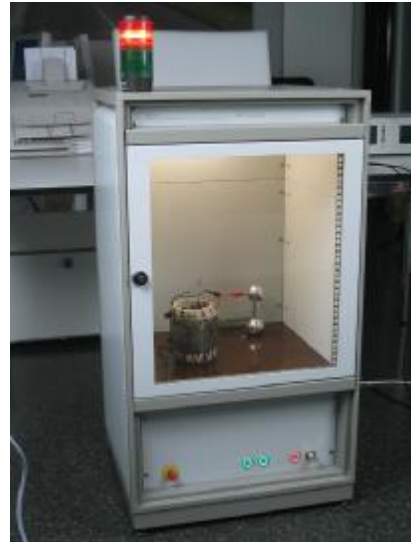
Partial discharge test cabinet for stator coils of small induction motors
