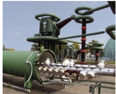
ATTanalyzer monitors a long-term test on GIS spacers and insulators (SIEMENS)
