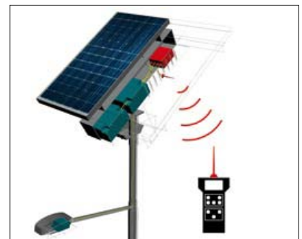
monitoring by remote control (max. 15 meters)
