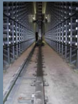
PosiTrack's 0.8 mm accuracy is ideal for horizontal pick-and-place feedback in automated storage and retrieval systems.
