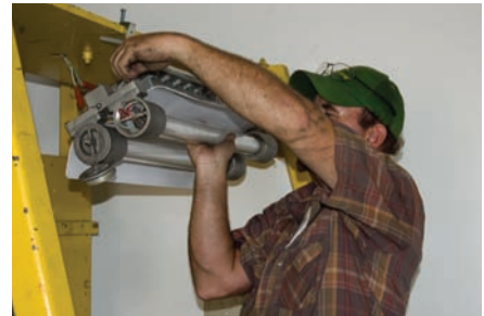
3. While supporting the globe end casting, loosen and remove the 4 bolts from each end.
