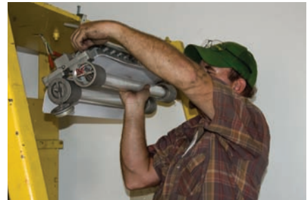
3. While supporting the globe end casting, loosen and remove the 4 bolts from each end.
