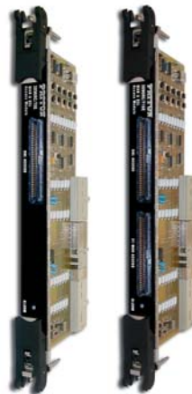
Rear transition modules with flexible interface capabilities
