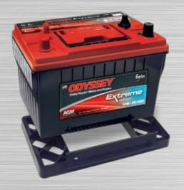
Optional height adapter may be used on the 34M-PC1500 for installations where a group 24 or group 27 is required. Snap the adapter securely into place on the bottom of the 34M-PC1500 battery. In some installations, a 34M-PC1500 with this adapter may be used to replace a group 24F or 27F depending on required cable length.
