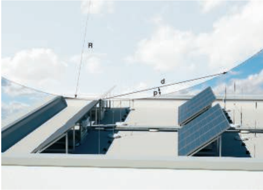
Figure 1: Planning method: Rolling sphere ( R ), rolling sphere method and penetration depth ( p ) and spacing of the interception rods ( d )
