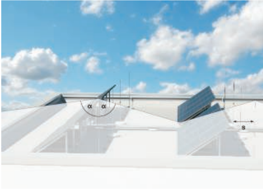
Figure 2: \alpha^\circ = Lightning protection angle
