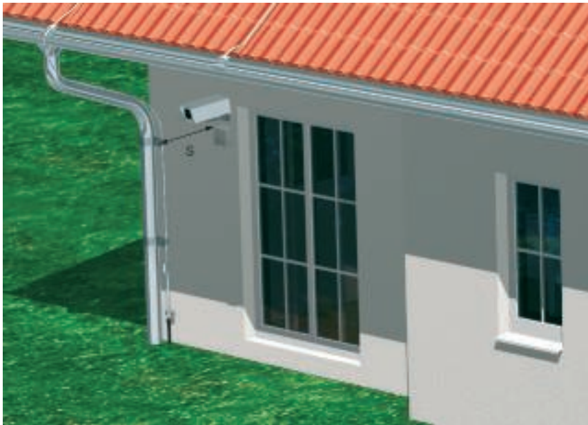
Correctly observed separation distance (s) between arrestor equipment and camera
