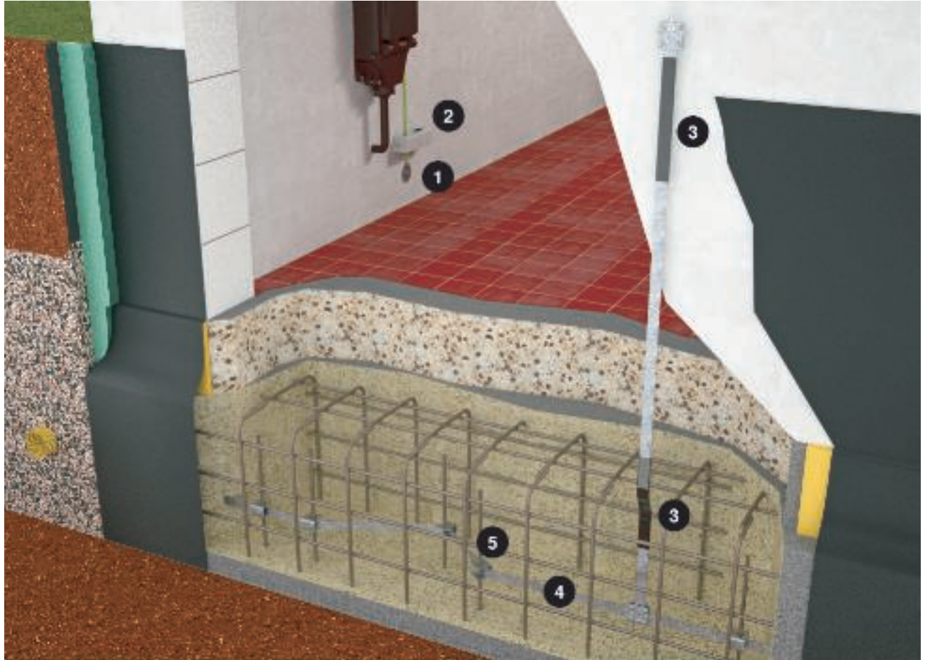
1 = Earthing fixed point, 2 = Equipotential bonding rail, 3 = Corrosion protection strips, 4 = Cable material, 5 = Connection terminals
