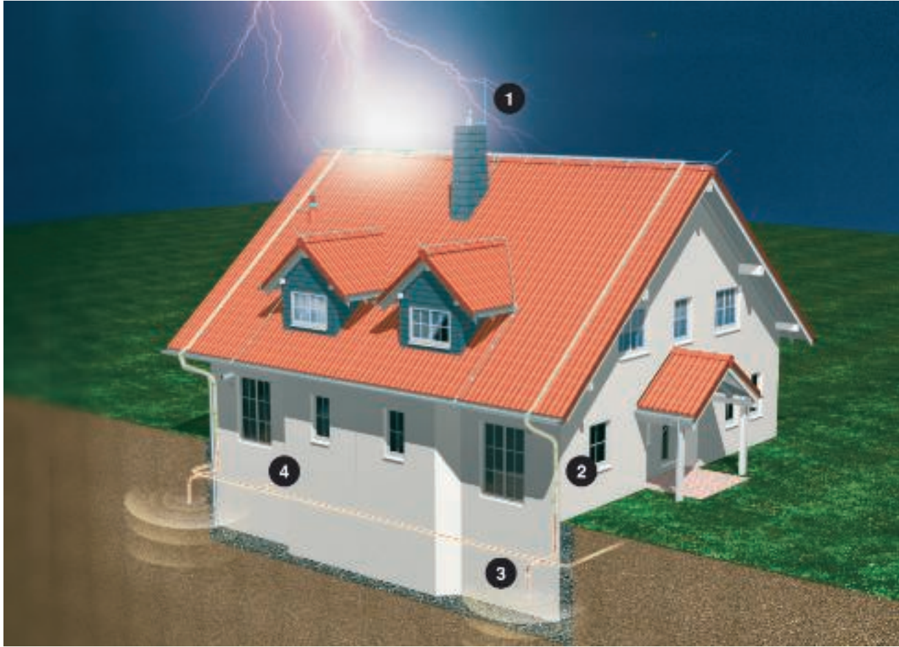
1 = Interception unit, 2 = Arrestor, 3 = Earthing system, 4 = Equipotential bonding
