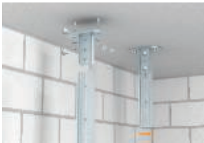
Head plate mounting Fastening of the standard head plate, KI 8, for I support to concrete ceilings using anchor bolts, type FAZ II.
