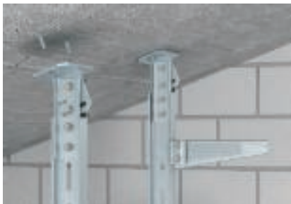
Head plate, variable (rotated through 90°) Installation of the variable head plate, rotated through 90°, KI 8 VLK to sloping concrete ceilings using anchor bolts, type FAZ II.
