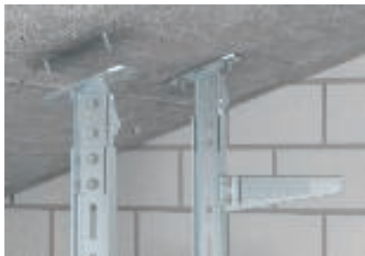
Variable head plate Installation of the variable head plate KI 8 VQP to sloping concrete ceilings using anchor bolts, type FAZ II.
