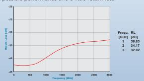
The higher the frequencies the more pronounced is the "skin effect", which means the energy moves to the outside of the conductor. Therefore the plating of outer and center contact is more important than on audio connectors with low frequencies - both contacts of our BNC connectors are gold plated.
