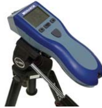
PLT200 and PT99 have a 1/4" 20 threaded bushing for tripod mounting
