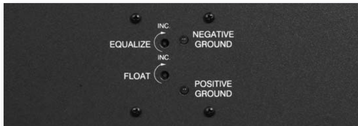
Ground Detection LED's (46J, 46Q, 46T & 46U only) shown on A12B model
