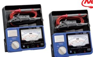
IR4016-20, 4017-20, 4018-20 €€ Single range IR4016-20: 500V/100MΩ IR4017-20: 500V/1000MΩ IR4018-20: 1000V/2000MΩ Compact and lightweight, Luminous scale indicator type ..... p.61
