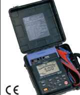
3455 €€ Testing voltage 250V to 5000V, Five ranges 10 MΩ to 5 TΩ Seven ranges ..... p.59
