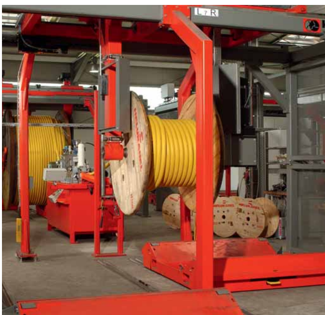
Heavy-load, cable-cutting facility
