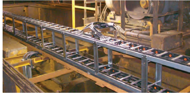
Gortrac designed high velocity Rolling Carriage with plastic TS carrier for long travel in a steel mill.
