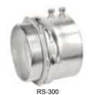
**Application:** These set-screw connectors are used in dry locations to bond unthreaded rigid or IMC conduits to electrical junction boxes or electrical enclosures. Garvin Industries' steel set-screw connectors provide concrete-tight connections when taped.
