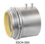
Application: These insulated electrical connectors are used in dry locations to bond EMT thinwall conduits to electrical junction boxes or enclosures. Garvin Industries' insulated, steel set-screw connectors provide concrete-tight connections when taped and properly secured with the included locknut. They are rated for electrical applications above 600 volts
