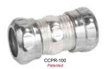
**Application:** These rain-tight compression couplings are used in wet locations to connect the ends of two EMT thinwall conduits together to extend the raceway. Garvin Industries' rain-tight steel EMT compression couplings have been designed to comply with the new rain-tight test requirements along with the 2008 NEC 358.42 and 314.15 requirements.
