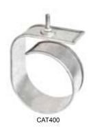
**Application:** These looped cable support harnesses are versatile and can be attached to a wide variety of structures using beam clamps, clips and other support components available from Garvin Industries. These support harnesses eliminate the problem of point loads that can cause cable damage to sensitive cables such as fiber optic cables CAT 5E, 6, 7, etc.
