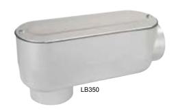
**Application:** Conduit bodies are attached to threaded rigid or IMC conduits when a change of direction is required. Removable cover and gasket allow for easy wire pulling and feed through. Commonly used for electrical service entrance wires or as an economical convenience box when extra wire space is needed.
