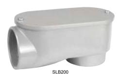
**Application:** Conduit bodies are attached to threaded rigid or IMC pipe in opposite directions. Removable cover and gasket allow for easy wire pulling and feed through. Commonly used for electrical service entrance wires or as an economical convenience box when extra wire space is needed.
