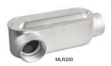
**Application:** Conduit bodies are attached to threaded rigid conduits when a turn is required and conduit bending is not convenient or possible. Removable cover and gasket allow for easy wire pulling and feed through. Commonly used as an economical convenience box when extra wire space is needed.
