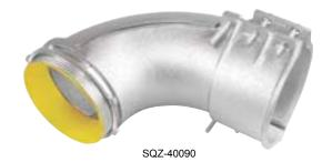
Application: These 90 degree squeeze type connectors with insulated throats are used in dry locations to bond flexible metal conduits to boxes or enclosures.
