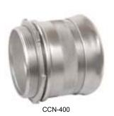
Application: These uninsulated compression connectors are used to bond EMT thinwall conduits to electrical junction boxes or enclosures. Garvin Industries' uninsulated, steel compression connectors provide concrete-tight connections when taped, and are rated for electrical applications above 600 volts.
