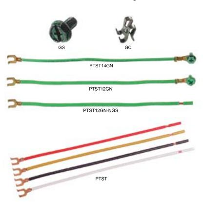
Application: These box grounding accessories aid in safe electrical grounding path to help prevent any electrical shock. Grounding screws thread into boxes and provide a means of fastening the ground conductors. Grounding wires fasten into the boxes and are then connected to wiring systems or devices. Grounding clips provide an easy method of fastening grounding conductors to the edges of steel outlet boxes.
