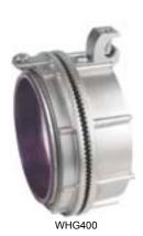
**Application:** These watertight hubs with grounding lugs are used to secure threaded rigid or IMC conduits to electrical boxes or enclosures. They have insulated throats to protect wires from damage.
