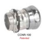
**Application:** These rain-tight compression connectors are used in wet locations to bond EMT thinwall conduits to electrical junction boxes or enclosures. Garvin Industries' rain-tight EMT compression connectors have been designed to comply with the new rain-tight test requirements along with the 2008 NEC 358.42 and 314.15 requirements.
