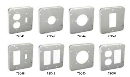
**Application:** These 1/2" raised surface covers with included screws and nuts are used to mount electrical devices on 4-11/16" square boxes in industrial settings. They are also used when boxes are surface mounted or positioned in exposed work applications.
