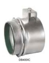
**Application:** These saddle connectors are used on flexible metal conduits, armored clad cables and metal clad cables. Their dual-grip saddle and quick screw tightly fit on flexible metal cables ensuring the metal jacket will not be damaged or distorted protecting the wires.
