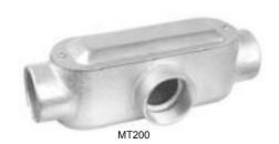
Application: Conduit bodies are attached to threaded rigid conduits when a turn is required and conduit bending is not convenient or possible. Removable cover and gasket allow for easy wire pulling and feed through. Commonly used as an economical convenience box when extra wire space is needed.
