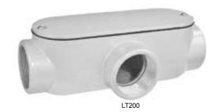
**Application:** Conduit bodies are attached to threaded rigid or IMC conduits when a change of direction is required. Removable cover and gasket allow for easy wire pulling and feed through. Commonly used as an economical convenience box when extra wire space is needed.
