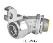
**Application:** These 45° connectors with insulated throats and grounding lugs are used in both indoor and outdoor locations on flexible metallic, liquid-tight conduits when copper or aluminum jumper installations are required.
