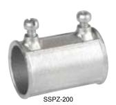
Application: These set-screw couplings are used in dry locations to connect the ends of two EMT thinwall conduits together. Garvin Industries' die-cast zinc, set-screw couplings provide concrete-tight connections when taped and properly secured with the included set-screw. Garvin Industries' set-screw electrical couplings are rated for electrical applications above 600 volts.
