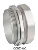
**Application:** These uninsulated compression connectors are used in dry locations to bond EMT thinwall conduits to electrical junction boxes or enclosures. Garvin Industries' uninsulated compression connectors provide concrete-tight connections when taped and properly secured with the included locknut. Garvin Industries' uninsulated compression connectors are rated for electrical applications above 600 volts.
