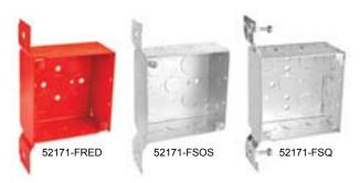
**Application:** These bracket boxes with conduit knockouts are used when 4" square boxes must be mounted directly to wood or metal studs. Square boxes are used to bring power to a number of electrical devices where multiple conductor runs are split in two or more directions.
