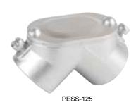
**Application:** These set-screw EMT pull elbows are used when 90° turns are needed in conduits and when wires must be pulled through elbows before making the turn. Their removable gasket and cover allow for wires to be pulled and fed back into pipes at a 90° angle or turn.
