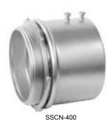
**Application:** These uninsulated electrical connectors are used in dry locations to bond EMT thinwall conduits to electrical junction boxes or enclosures. Garvin Industries' uninsulated, steel set-screw connectors provide concrete-tight connections when taped and properly secured with the included locknut. They are rated for electrical applications above 600 volts
