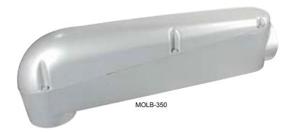
Application: Mogul conduit bodies are attached to threaded rigid conduits when a change of direction in the conduit run requires wires to be pulled and fed through in a new direction. Removable cover and gasket allow for easy wire pulling and feed through. Commonly used for electrical service entrance wires or as an economical convenience box when extra wire capacity is needed.
