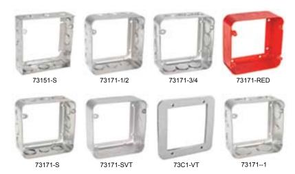
**Application:** These extension rings with conduit knockouts are added to junction boxes to increase wiring capacity and provide access for additional conduit runs.
