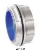
**Application:** These watertight hubs are used with threaded rigid or IMC conduits to connect and bond them to threaded openings in boxes or enclosures. Garvin Industries' die-cast zinc, watertight hubs may be used in both wet and dry locations
