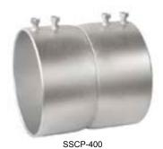
**Application:** These electrical couplings are used in dry locations to connect the ends of two EMT thinwall conduits together to extend the raceway. Garvin Industries' steel, setscrew couplings provide concrete-tight connections when taped and properly secured with the included set-screws. These steel set-screw couplings are rated for electrical applications above 600 volts.
