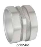
**Application:** These electrical compression couplings are used to connect the ends of two EMT thinwall conduits together to extend the electrical raceway. Garvin Industries' compression couplings provide concrete-tight connections and are rated for electrical applications above 600 volts.
