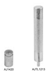
Application: These expansive, screw anchors are used in walls to provide a threaded wall insert for mounting various boxes, hangers and straps. They are not to be used in ceilings. Lead anchor set tools are used to forcibly strike threaded anchors and set them in pre-drilled holes. Striking the anchors causes them to expand, securely wedging them in walls. When bolts and screws are inserted they further expand the anchors, providing a sturdy, secure fastening point on solid walls.
