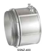
Application: These uninsulated set-screw connectors are used in dry locations to bond EMT thinwall conduits to electrical junction boxes or enclosures. Garvin Industries' uninsulated, die-cast zinc, set-screw connectors provide concrete-tight connections when taped and properly secured with the included locknut. Garvin Industries' set-screw electrical connectors are rated for electrical applications above 600 volts.
