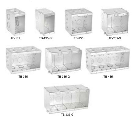
**Application:** These masonry boxes are used for mounting switches, plugs, outlets and other electronic and electrical devices in masonry, brick and block walls. The Gangable versions offer installers the ability to add devices in the field. Use 2-1/2" deep boxes in 4" block walls. Use 3-1/2" deep boxes in 6" or 8" walls.
