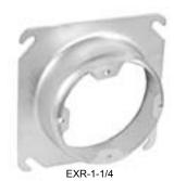
**Application:** These dual-direction, square-to-round device covers are mounted on ceilings or walls for proper alignment of any device or fixture with canopy installed. Typically used on exit signs, emergency lights, ceiling fixtures, security cameras, wall sconce lights and electronic devices.
