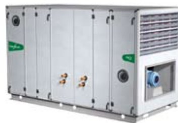
Supply air and exhaust air unit with rotary or plate heat exchanger. All components built in, such as fans, filters, dampers, heat exchanger, cooling and heating coils.
