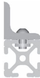
Slide pre-loaded part into T-slot
