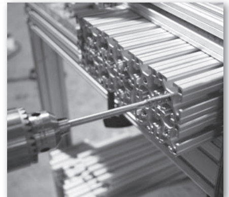
Tap services are per end of extrusion
