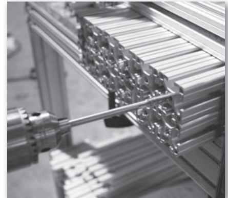
Tap services are per end of extrusion
