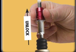
Move red ring up to unlock bit
