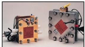
ElectroChem, Inc.'s fuel cell consists of a Nafion<sup>™</sup>-based MEA (manufactured by ElectroChem, Inc.) sealed between two gaskets mounted in between two graphite plates with a current collector plate on both ends.
