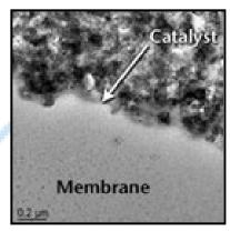
Atypical Pt catalysts for fuel cell applications contain 10%,20%,40% or 60% Pt on VULCAN XC-72R carbon support. Typical Electrochemical Area (ECA) for 20% Pt/C is  $100 \text{ m}^2/\text{q}$ . Typical ECA for 10% Pt/C is  $140 \text{ m}^2/\text{q}$ .
