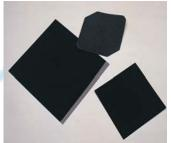
in PAFC and PEM membrane electrode assemblies as well as in different types of batteries. We use Platinum/Carbon catalyst with various loadings laminated to a hydrophobic GDL.
