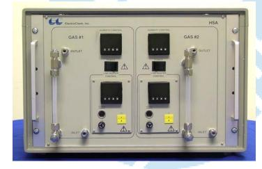
The HSA™ humidifier unit is used to provide humidification to two reactant gas supply lines for the electrochemical testing of PEM, alkaline, and phosphoric acid fuel cells. It provides enough capacity for single cells and fuel cell stacks. This unit is often used to support the
