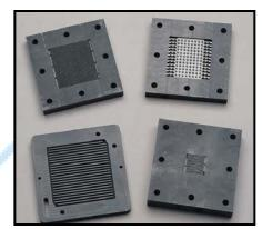
The purpose of the flow field on the graphite separator plates is to establish uniform distribution and pressure drop of reactants across the fuel cell and to remove the product water/gas.
