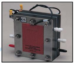
Current is collected by connection to copper contact plates; separate voltage connectors are provided directly in the cellblocks for maximum accuracy in iR measurement. Each unit includes resistive heaters and thermocouple wells for accurate temperature control.
