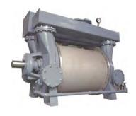
Edwards offers a full range of liquid ring pumps. The LR1A19000 provides a single-stage design and curved blade impellor with reinforcing rings for improved ruggedness, reducing noise and vibration.
