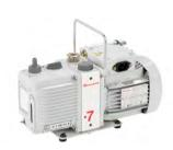
The E2M0.7 is a small two stage oil sealed rotary vane pump that features a very low sound level of only 43 dB(A), compact dimensions, low energy consumption and low operating temperature. It will appeal to scientific instrument manufacturers and laboratory users for backing small turbomolecular or diffusion pumps as well as general laboratory applications.
