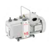
The E2M1.5 is a two stage oil sealed rotary vane pump suitable for many bench type applications. The pump features an alternative inlet connection position at the side of the pump so that overall installation height can be reduced to a minimum when required.
