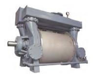
Edwards offers a full range of liquid ring pumps. The LR1B8000 provides a single-stage design and curved blade impellor with reinforcing rings for improved ruggedness, reducing noise and vibration.
