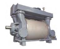
Edwards offers a full range of liquid ring pumps. The LR1B15000 provides a single-stage design and curved blade impellor with reinforcing rings for improved ruggedness, reducing noise and vibration.
