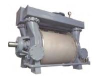
Edwards offers a full range of liquid ring pumps. The LR1A26000 provides a single-stage design and curved blade impellor with reinforcing rings for improved ruggedness, reducing noise and vibration.
