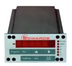
The Model 1575 Pressure Display is a low cost, microprocessor based, digital display and set-point controller for the Barocel 600, 622 and 655 capacitance manometers. The Model 1575 incorporates power supply, digital display, four user-selectable set-points, along with analog outputs in a compact 1/8 DIN package.
