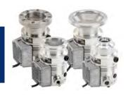
The EXT75DX compound turbomolecular pumps combine the proven technology of a ceramic mechanical lower bearing, a dry permanent magnetic upper bearing and Holweck drag stage with the added convenience of an on-board 24V controller allowing parallel and serial communication compatible without TIC controllers.
