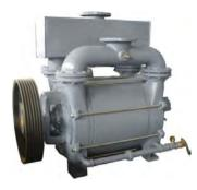
Edwards offers a full range of liquid ring pumps. The LR1A800 provides a single-stage design and curved blade impellor with reinforcing rings for improved ruggedness, reducing noise and vibration.
