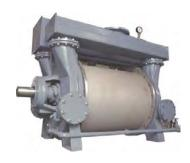
Edwards offers a full range of liquid ring pumps. The LR1B4500 provides a single-stage design and curved blade impellor with reinforcing rings for improved ruggedness, reducing noise and vibration.
