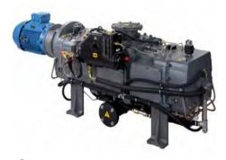
The Drystar® GV80 – 600M range is based on the well proven Edwards reverse claw mechanism reaching a peak speed of 560  $\rm m^3h^{-1}$  / 330  $\rm ft^3min^{-1}$ . The reverse claw mechanism results in short gas paths within the operating mechanism, providing the ability to handle large amounts of dust and water vapor, when compared to oil sealed pumps, without deterioration of performance.
