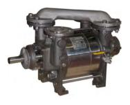
Pumps can be supplied as bareshaft or as part of a package complete with drive motor, discharge separator, heat exchanger and other accessories for recirculation of the seal liquid. In addition, all Edwards liquid ring pumps are available as part of ATEX category 1 or category 2 pump systems.
