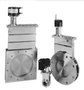
The Edwards GV range of stainless steel bellows sealed gate valves are designed for applications requiring overall leak tightness and a minimum of hydrocarbon in the residual atmosphere. These superior quality valves offer high vacuum integrity coupled with maximum conductance.
