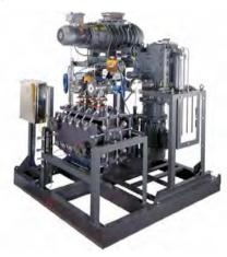
The proven and rugged non contacting designs, both screw and reverse claw mechanisms, include the ability to control pump body and internal gas temperatures allowing a comprehensive range of solvents, flammables and corrosives to be pumped. Systemized variants address the EU's explosive atmospheres (ATEX) directive for Category (Zone 0) T4 operation. The mechanisms are both highly tolerant to liquids and particles in the gas stream and are suitable for many applications, including:
