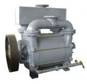
Edwards offers a full range of liquid ring pumps. The LR1A300 provides a single-stage design and curved blade impellor with reinforcing rings for improved ruggedness, reducing noise and vibration.
