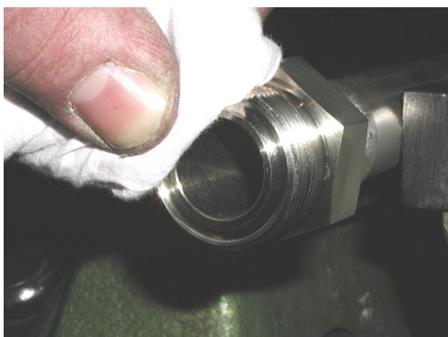
7. Before assembling clean the DILO tongue and groove
