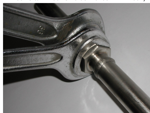
10. Tighten fast and strongly (pay attention to the torque) the clamping nut by counteracting force
