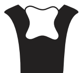
Type B - Same dimensions as the Deep seal. Beveled lip design provides better film breaking. Utilizes type "B" lip. Typical Part Number U25-2.50-37B
