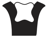
Type SQB - Same dimensions as the Standard seal. Beveled lip design provides better film breaking. Utilizes type "B" lip. Typical Part Number U25-2.50-SQB
