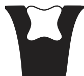
Deep - Utilizes the same "D" lip, but the seal height is greater than the cross section, thus giving a rectangular shape. Typical Part Number U25-2.50-37D
