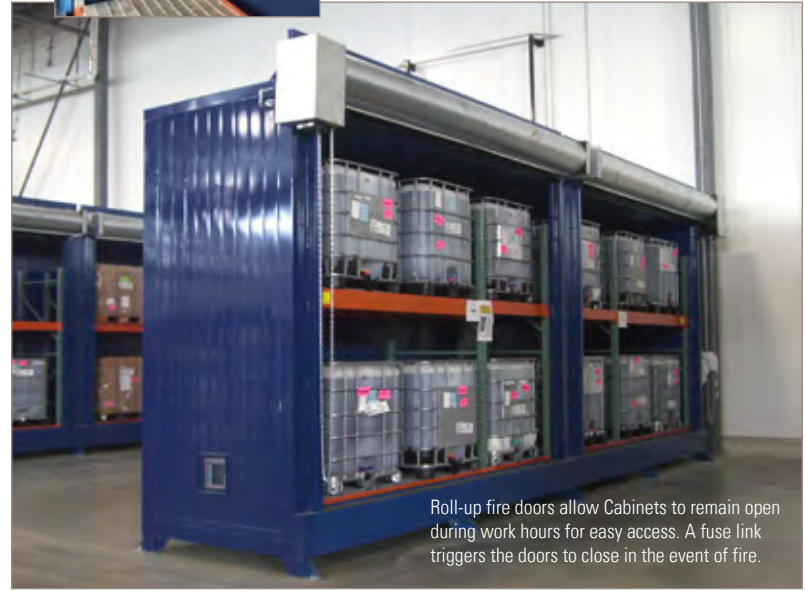
Single tiered unit provides storage for either eight 55 gallon drums or two 350 gallon totes
