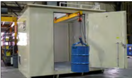
A crane system to ease drum handling
