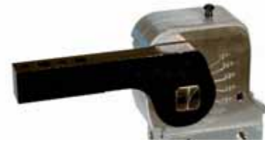
Lateral clamping arm, horizontal clamping position
