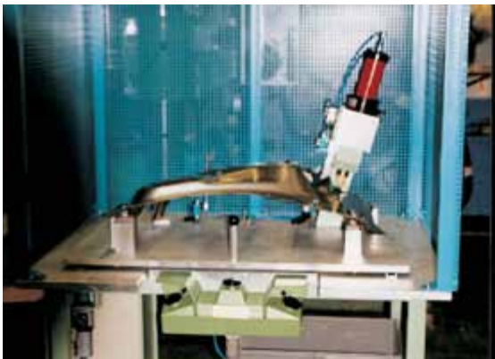
Device for holes Ø 8 in sheet metal
