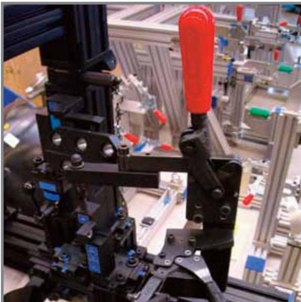
Model 533-LB and 227-UB shown with black finish in a fixture for used for optical inspection.
