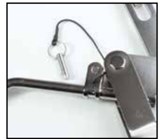
Redesigned Positive Locking Closure with Quick Pin
