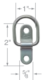
3/16" Hinged Pad Eye Safe Working Load: 400 lbs
