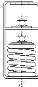
Option 3 Furnished with a positioning plate to hold equipment at a fixed elevation during installation.
