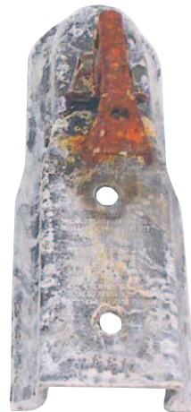
Competitor's coupler after 336 hours salt spray testing.
