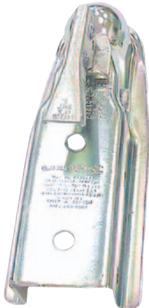
Fulton coupler after 336 hours salt spray testing.
