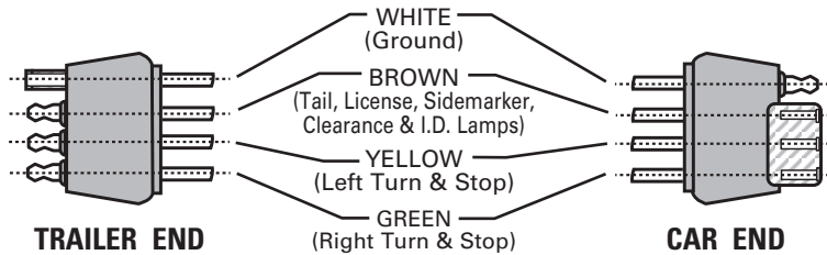
TRAILER END As viewed from core back side where wires are attached with screws.
