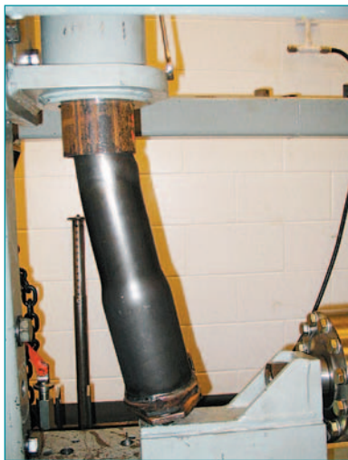
Competitor's 25K gooseneck fails longitudinal test at 11,500 lbs.
