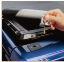
Removable eyelet for a flush mounting system
