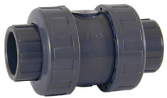
PVC TRUE UNION 4 O-rings: EPDM 150 psi @ 73°F
