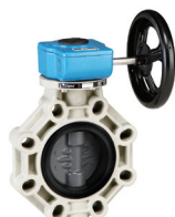
PPL - GF with gear box Stainless steel stem (AISI 630) PVC valve disc O-rings: Viton® 150 psi @ 73°F
