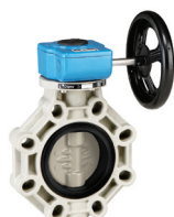
PPL - GF with gear box Stainless steel stem (AISI 630) PPL valve disc O-rings: Viton® 150 psi @ 73°F
