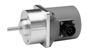
Celesco's model RT8420 provides extended rotational position feedback from as little as 1/8 of a turn f.s. all the way up to 200 turns f.s. The RT8420 combines the superb linearity and resolution of a plastic-hybrid potententiometer with the durability of Celesco's 4...20 mA circuit to provide an accurate and reliable electrical signal over all ranges.
