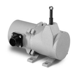
The PT8510 can operate from an unregulated 14.5 to 40 VDC power supply while providing an output signal that is proportional to the linear movement of it's measuring cable. The PT8510 has a maximum measurement range up to 60" and has 4 output signal options to choose from: 0...10, 0...5, -10...+10 and -5...+5 Vdc.
