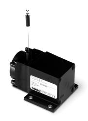
The PT1MA adds 4...20 mA position feedback signal to Celesco's compact line of cable-extension transducers. The PT1MA is available with full stroke ranges from as little as 2 inches on up to 50 inches with adjustable zero and span settings to precisely match the full scale output to your exact measurement range.
