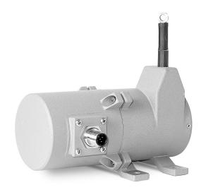
The PT8DN, using a high cycle plastic-hybrid potentiometer, communicates via DeviceNET protocol with programmable controllers in factories and harsh environments requiring linear position measurements in ranges up to 60".
