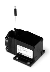
The heart of the PT1E is an incremental optical encoder which delivers a quadrature formated digital pulse train. This compact transducer is available with several resolution options for a wide variety of applications from high accuracy position feedback to slow velocity feedback requirements.
