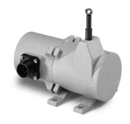
The PT8101, using a high cycle plastic-hybrid potentiometer, operates with any basic panel meter or programmable controller in factories and harsh environments requiring linear position measurements in ranges up to 60".
