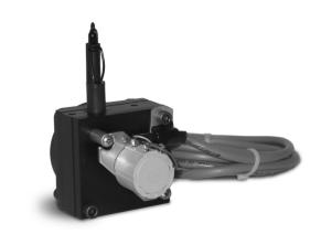
The PTX101 is a low cost, compact and easy-to-use cable-extension transducer. It is available with full-scale measurement ranges from 2 to 100 inches. The PTX101 provides a voltage feedback signal that is proportional to the linear movement of a traveling stainless-steel extension cable.
