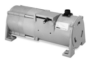
The PT9301 is a combination position and velocity transducer for demanding long-range applications requiring a linear position measurements in ranges up to 1700". A precision plastic-hybrid potentiometer provides accurate position feedback while a self-generating DC tachometer provides a velocity signal that is proportional to the speed of the traveling stainless-steel measuring cable.
