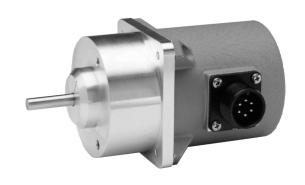
The RT8510 can operate from an unregulated 14.5 to 40 VDC power supply while providing a regulated output signal over it's full range from 1/8 of a turn up to 200 turns. It provides a 0 - 10 VDC position feedback signal proportional to the rotational position of the shaft
