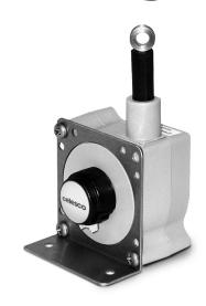
The Celesco SE1 is the digital encoder version of our compact String Pot series. The SE1 is an economical and durable device that utilizes a flexible cable, a spring-loaded spool and an incremental optical encoder to detect and measure linear position.
