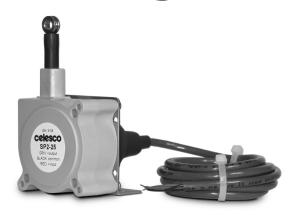
The SP2 String Pot from Celesco is a compact, economical and water resistant device that utilizes a flexible cable, a spring-loaded spool and a potentiometer to detect and measure linear position.
