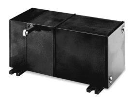
The PT5AV is a combination position and velocity transducer. A precision plastic-hybrid potentiometer provides accurate position feedback while a self-generating DC tachometer provides a velocity signal that is proportional to the speed of the traveling measuring cable.
