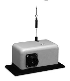
The PT420 is available with full-scale measurement ranges from 2 to 100 inches, providing a 0/4-20 mA feedback signal that is linearly proportional to the position of a traveling stainless-steel extension cable. Use the PT420 to provide position feedback on hydraulic cylinders in factories and utilities, gate position in fresh or wastewater distribution systems, or valve opening in process-related applications.
