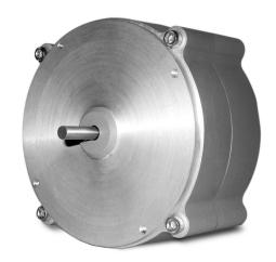
Celesco's model RT9CN communicates rotational position feedback to your PLC via the CANbus SAE J1939 interface. The heart of this sensor is a precision plastic-hybrid position potentiometer which provides a "absolute" position and does not ever have to be reset to a "home" position after a power loss or planned shutdown.
