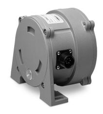
The IT9232 delivers incline position feedback via RS232 serial communication to your data acquisition or controller system. The heart of this inclinometer is a magnetically-damped pendulum coupled to a conductive plastic precision potentiometer.
