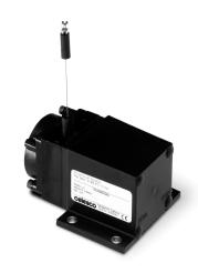
The PT1DC can operate from an unregulated 14.5 to 40 VDC power supply while providing an output signal that is proportional to the linear movement of it's measuring cable. The PT1DC has a maximum measurement range up to 50" and has 4 output signal options to choose from: 0...10, 0...5, -10...+10 and -5...+5 Vdc.
