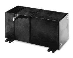
The PT5232, delivers position feedback via RS232 serial communication to your data acquisition or controller system. The PT5232 sends a raw 16-bit position count from 0000 to FFFF (hex). Additionally this device can be set to continuously send data or send data only when polled.
