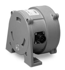
The model IT9101 is a rugged and simple device which provides a voltage divider feedback signal for incline position. The heart of the IT9101 is a magnetically-damped pendulum coupled to a conductive plastic precision potentiometer.
