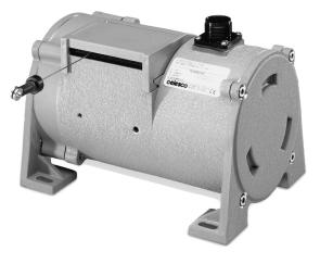
The PT9301 is a combination position and velocity transducer for demanding long-range applications requiring a linear position measurements in ranges up to 1700". A precision plastic-hybrid potentiometer provides accurate position feedback while a self-generating DC tachometer provides a velocity signal that is proportional to the speed of the traveling stainless-steel measuring cable.
