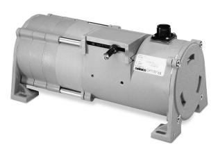
The PT9232 delivers position feedback via RS232 serial communication to your data acquisition or controller system. The PT9232 sends a raw 16-bit count from 0000H to FFFFH. Additionally this device can be set to continuously send data or send data only when polled.
