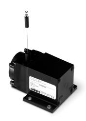
The PT1A is perfect where space and money are limited. The PT1A is part of Celesco's compact line of cable-extension transducers. Using a high cycle plastic-hybrid potentiometer, the PT1A provides a precision voltage divider position feedback signal for full-scale measurement ranges from 2 to 50 inches.
