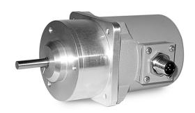
Celesco's model RT8CN communicates rotational position feedback to your PLC via the CANbus SAE J1939 interface. The heart of this sensor is a precision plastic-hybrid position potentiometer which provides a "absolute" position and does not ever have to be reset to a "home" position after a power loss or planned shutdown.
