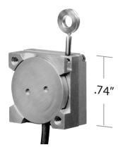
Introducing the world's smallest stringpot. The M150 is smaller than a thumbprint and occupies a tiny space of only .74 x .74 x .38 inches. With a full stroke measurement range of 1.5 inches, the M150 has been designed for many aerospace and automotive space-critical test applications such as throttle position and crash-test instrumentation.
