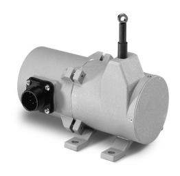
The PT8232 delivers position feedback via RS232 serial communication to your data acquisition or controller system. The PT8232 sends a raw 16-bit count from 0000H to FFFFH. Additionally this device can be set to continuously send data or send data only when polled.
