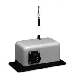
The DV301 is a combination position and velocity transducer for full-scale measurement ranges from 2 to 100 inches. A precision plastic-hybrid potentiometer provides accurate position feedback while a self-generating DC tachometer provides a velocity signal that is proportional to the speed of the traveling stainless-steel measuring cable.
