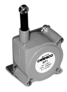
The Celesco SP1 String Pot is a compact, economical and durable device that utilizes a flexible cable, a spring-loaded spool, and a potentiometer to detect and measure linear position.
