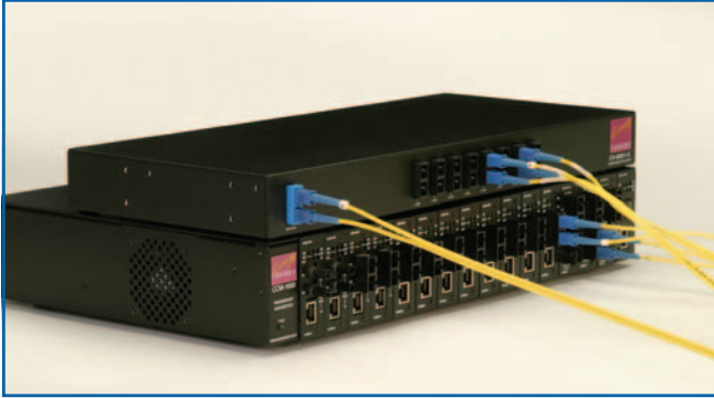
Illustrated: CCM-1600 Chassis connected to a CR-8MD1-E Standalone Multiplexer
