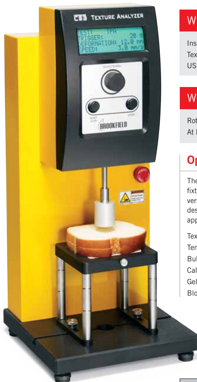
CT3 with Fixture Base Table and Cylindrical Probe in compression mode
