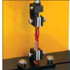
TA-DGA Dual Grip Assembly 5mm size shown
