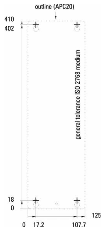
APC620 drilling template 3 full-size PCI slots
