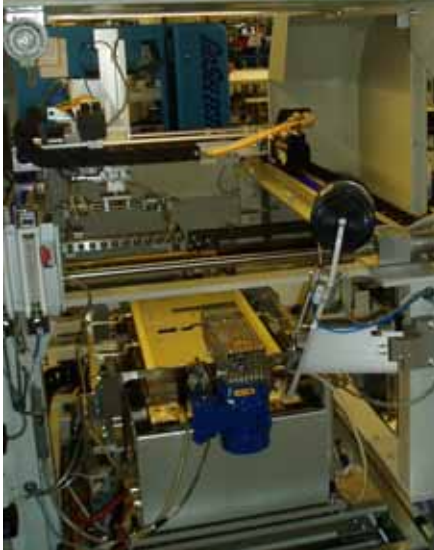
Selective soldering machine
