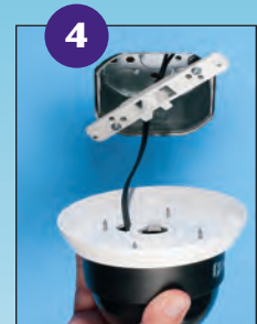
4 With camera mounted, install the mounting plate to the box by placing it on the bracket and turning clockwise to lock. Install set screw.
