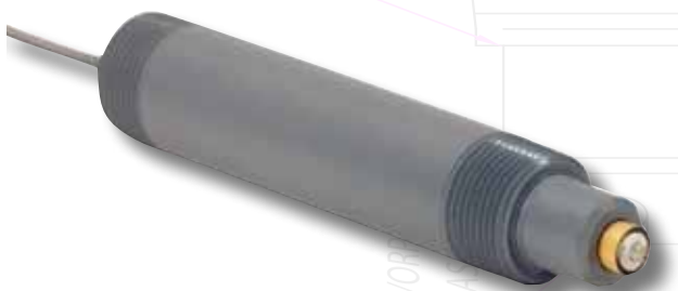
The P585 Combination probe is a combination glass electrode encapsulated in 3/4" epoxy body and comes with a 3/4" NPT compression fitting.
