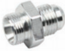
15207 Demon Carb AN-06 to 9/16" x 24 Thread Float Bowl Fitting
