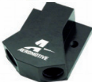
P/N 15620 High-Flow "Y" Block - (1) ORB-10 / (2) ORB-08
