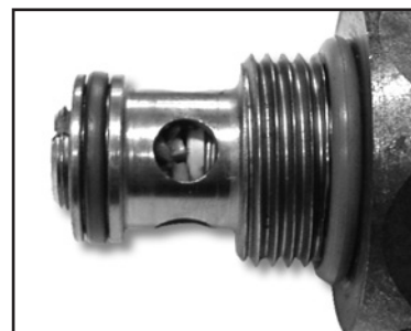
Blocked Modulating Valve
